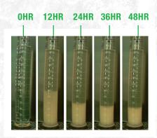
Wax crystals settling in standard cold flow improvers after 48 hours.
